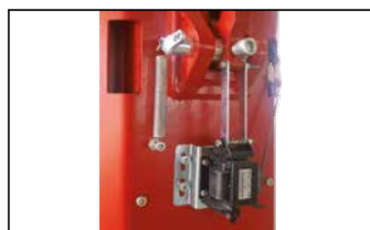
Electro magnet safety release 24V.
