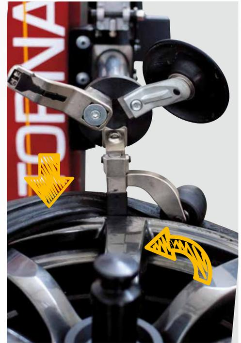
**E-F.** By positioning the REVOLVER mounting tool head between the rim and the tyre, the REVOLVER PLASTIC ROLLER will automatically help the tyre to stay in the channel.
