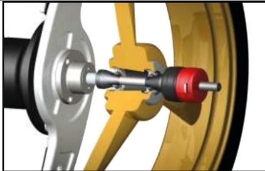
Shaft with centering cones.
